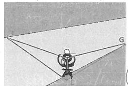
bank of the river and lowered the visor on his cap until the farthest thing visible was the edge of the bank on the other side. He then turned and noted the point on his side that was in line with the tip of his visor and his eye. The officer then paced to that point counting the distance from where the officer was to that point and concluded that distance was the width of the river. A) Explain how the officer came to his conclusion.
